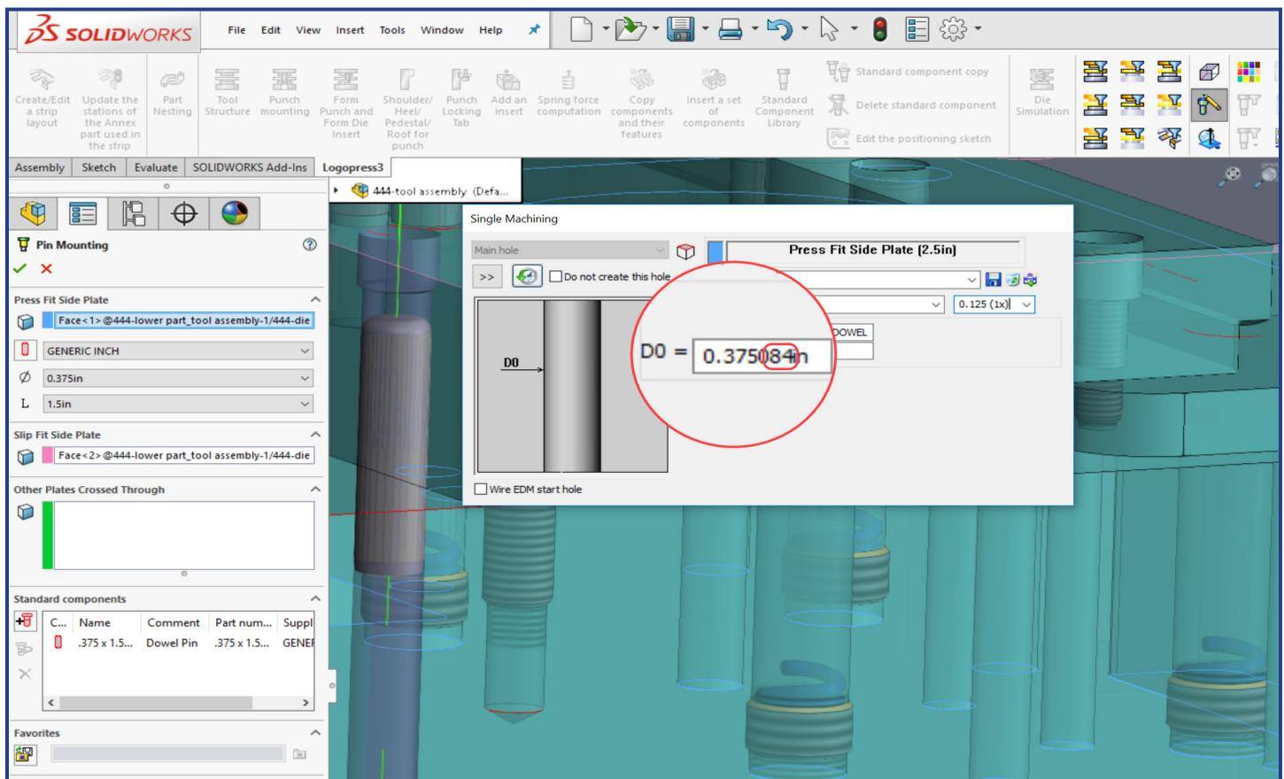
Trueline automatically conveys programming information to its 2.5-axis CAM software through specific decimal values in the values' 5th and 6th places that they have predefined within Logopress for each hole type, diameter, and component. This allows their rules-based CAM software to automatically determine what steps to take to machine each hole. Today, the company employs one programmer for four CNC mills and three CNC lathes.
