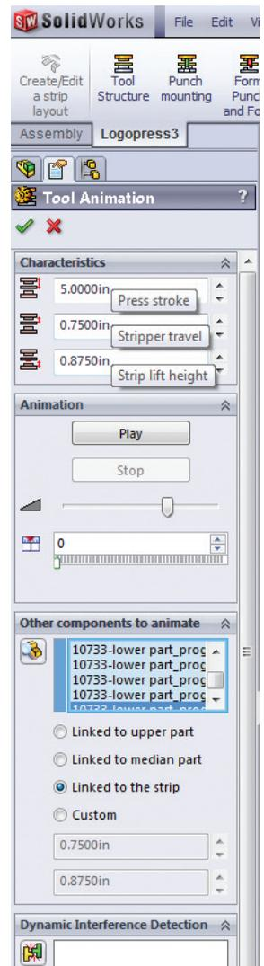
Because 3D design is much more visual, including the use of specialized tools for animating the die and performing dynamic interference detection, the task of training die designers is much less daunting.
