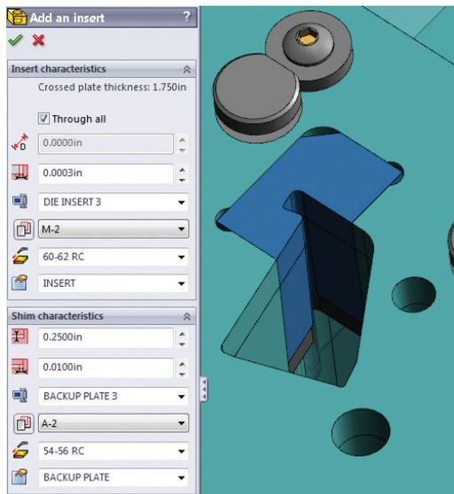
*In less than 5 min., an insert can be added to a plate along with a shim or backup plate, with proper clearances for both, along with various corner treatments for the cavity in the plate receiving the insert.*
