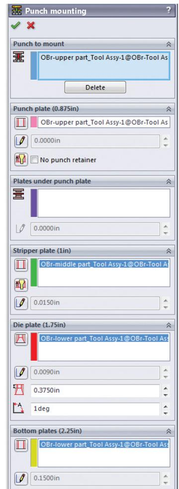
*The software will automatically cut all of the cavities through all plates in the die, applying the correct clearances and tapers.*
