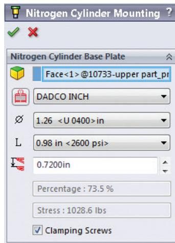
In the case of a nitrogen cylinder, the proper stroke length is automatically applied to the solid model of the cylinder; tonnage force is automatically calculated; the hole is cut for the cylinder and all plates it crosses through; and the screws that retain the cylinders are automatically created and inserted.
