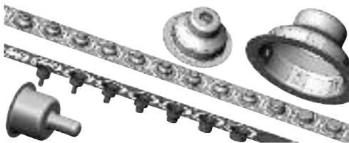
automatically handles stretch-web management. The program accounts for material characteristics as it automatically determines draw reductions.
