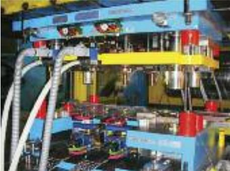
nected for applications where more than four elements are needed. The units, available for retrofit or installation in new progressive, transfer or tandem dies, can weld at press speeds to 60 strokes/min. The
