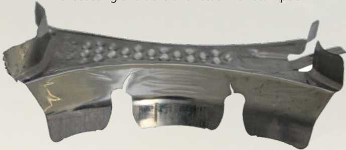
Heat shield with folds and cracks confirms simulation result
