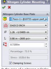
In the case of a nitrogen cylinder, the proper stroke length is automatically applied to the solid model of the cylinder; tonnage force is automatically calculated; the hole is cut for the cylinder and all plates it crosses though; and the screws that retain the cylinders are automatically created and inserted.
