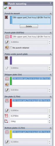
The software will automatically cut all of the cavities through all plates in the die, applying the correct clearances and tapers.
