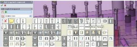
The die-design software includes a library of die components with multiple brands available for every component. The software automatically creates holes upon the insertion of the component, saving design time.
