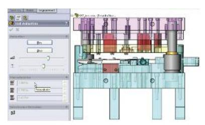
The Tool Animation command in the 3D die-design software employed at BesTech allows users to click an icon and then set the press stroke, stripper travel and strip-lift height. From there, animation shows the die running as if it were in the press. This feature also provides interference detection throughout the press stroke, including strip progression through the die.
